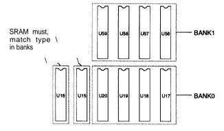
8KB or 32KB SRAM chips can be installed. Bank 0 must be filled before Bank 1. The SRAM type used for dirty RAM and tag RAM must match the type installed in the banks. The table below shows the possible configurations.
